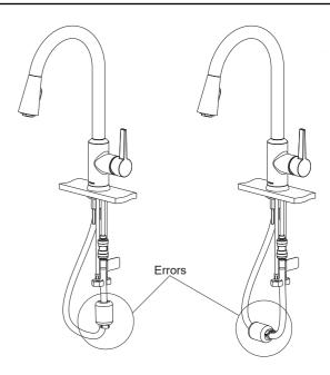
Put the weight(12) and clip(13) onto the pull hose(7). Connect the pull hose and the connecter(10). Adjust and position the weight and clip. **Note:** Don't over distort the hoses. Please avoid the wrong installation for the weight and clip as shown in the above.
